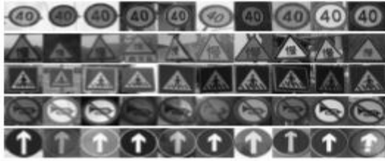
Figure 2: Traffic Signs coaching information Set. Traffic Signs Recognition and Classification supported Deep Feature Learning. Associate input sample with the dimensions of 48 \times 48 is convoluted with a 5 \times 5 convolutional kernel. Then, six 44 \times 44 feature maps square measure generated. Every somatic cell within the feature map is connected with 5 \times 5 hogged kernel. When the summation of every cluster of pixels within the feature map, the load and offset square measure added. When taking activate perform, the neurons within the next layer square measure mechanically non heritable. Naturally, following volume will be obtained by continuous translation and traverse operation.
