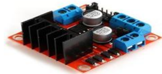
Fig 6. L298N Dual H Bridge DC Stepper Motor Drive Controller Board Module for Arduino
