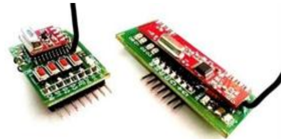
Fig 5. RF Transmitter & Receiver 433MHz with Encoder and Decoder
