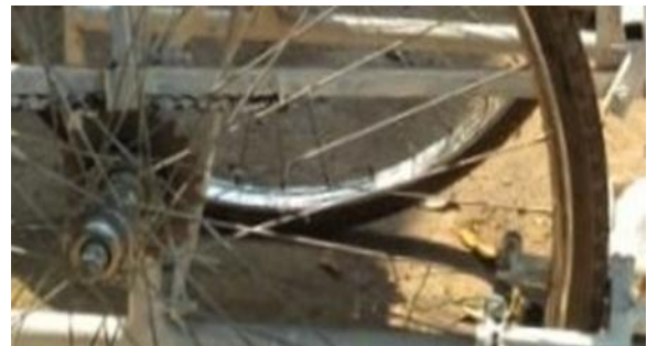
Fig 4.2.1: chain and sprocket use as rack and pinion
