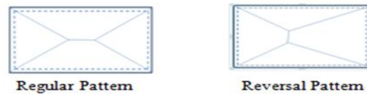
Fig.1 Rectangular Slab Yield Patterns
