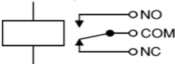
Fig.6. Relay Pins
