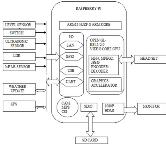
Figure 1: Block diagram for smart cane
