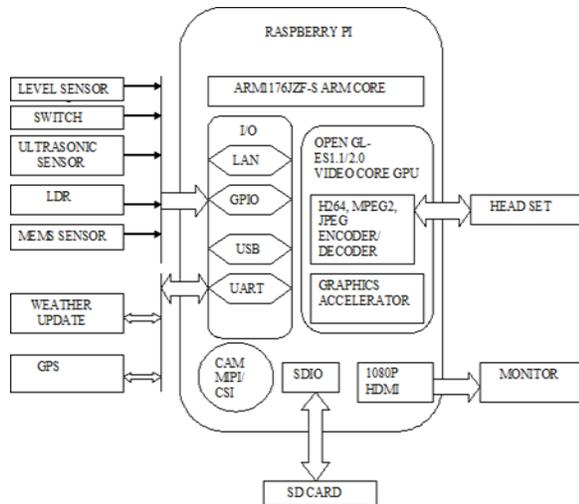
Figure 1: Block diagram for smart cane
