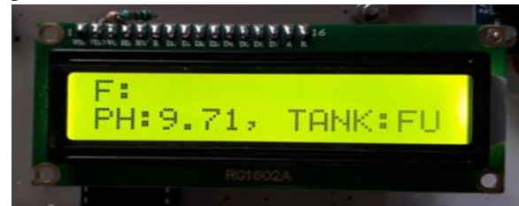
Fig. 9 LCD Output displaying the pH value and indicating that the tank is full.
