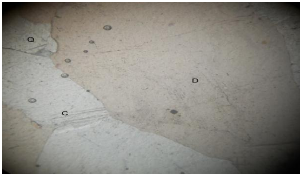
Figure 7: Photomicrograph of marble sample showing Calcite (C), Dolomite (D) (x40)
