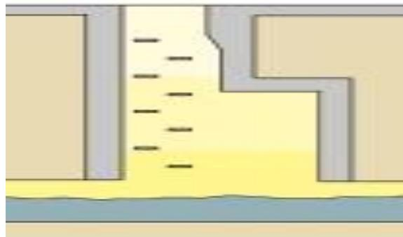
Different hazardous gases accumulate at different levels of a manhole
