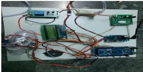
The hardware part of the system has the sensors which are attached to the mask. The oxygen tank is going to be given through the motor to the mask. Using an adapter and an influence supply the facility is given to the circuit. Relay circuit is employed for the motor. Wi-Fi module will update details to the online page and the LCD display will display the conditions of the sensors.
