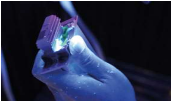
Fig. Liquid Penetrant test (Fluorescent Penetrant Inspection)
