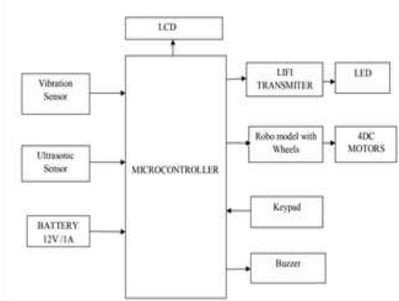
Fig 3: Transmitter Block Diagram
