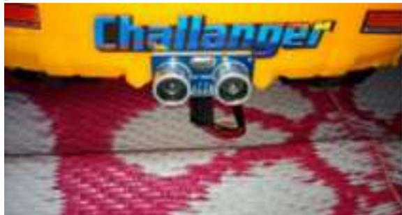
Fig 6: Ultrasonic Sensor
