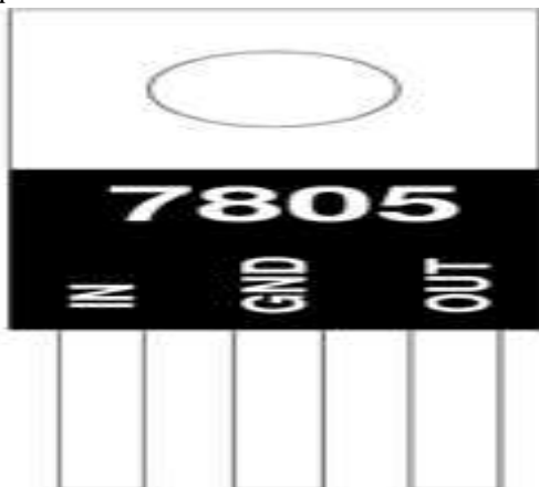
Figure : 7805 Voltage Regulator
