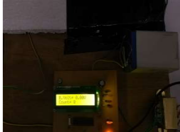
FIGURE: Initial reading on the display when no pressure is applied on the piezo sensors
