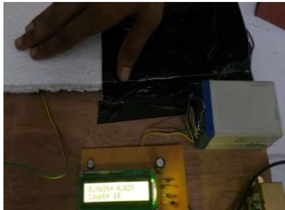
FIGURE: Voltage value and step count displayed when pressure is applied on the piezo sensors
