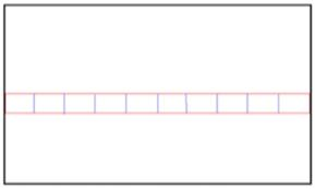
The count of white pixel in every unit in reference to black pixels is numbered respectively. This number determines the vehicle command.
