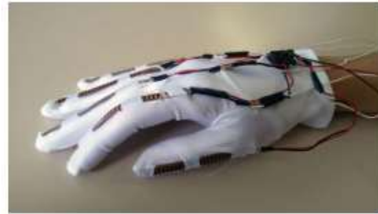
Figure 5. Control glove at the transmitter side Output voltage is measured by using a mathematical formula. This formula is a voltage divider formula (figure 6) using which, corresponding variable voltage will be measured which will be given as an input to the Arduino-UNO.
