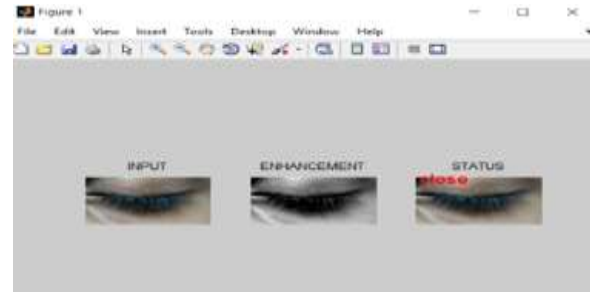
FIG.DROWSY DETECTION AFTER CLOSURE OF EYE
