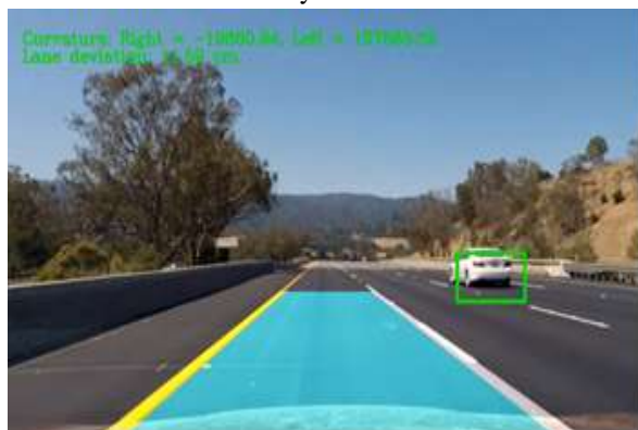
Fig. 5. Lane deviation, curvature and car tracking in video
