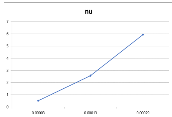
Fig 4.2. Variation of mass flow rate vs nusselt number of INLINE heat exchanger
