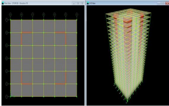
Fig.2- shear wall at interior of structure
