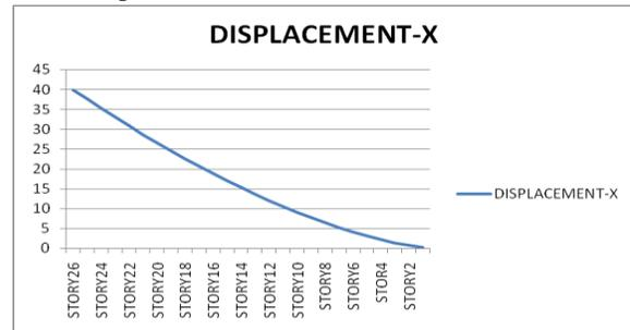
Fig.6: Maximum Displacement of structure
