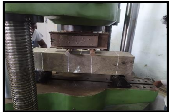
Two-point loading on conventional beam
