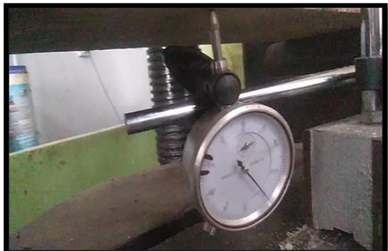
Deflection dial gauge for displacement measurement
