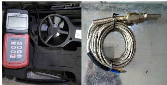
Fig1.3.- Anemometer Fig.1.4- J type thermocouple Fig.1.1 shows experimental setup from front view of 90° inlet. The baffles with straight angle and same
