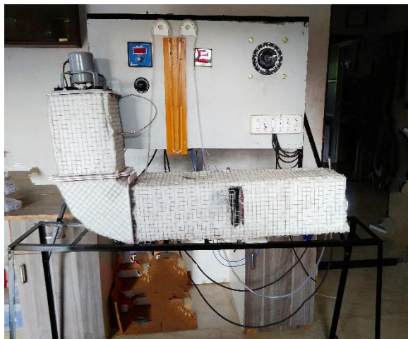
Fig.1.1- Actual Experimental Setup of Rectangular Channel 90° Inlet
