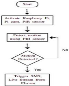
Once the device is switched ON, the Raspberry Pi, Pi cam and PIR sensors are activated. PIR sensors checks for any form of motion, if detect-ed SMS is trigged and LIVE STREAM from PI cam is turned on for the user to monitor the activities. For homes and offices, it is just not enough to have security guards. For 24\*7 surveillance, we require a closed-circuit television (CCTV) system. CCTV security system is an effective way and the perfect solution to the security problems.
