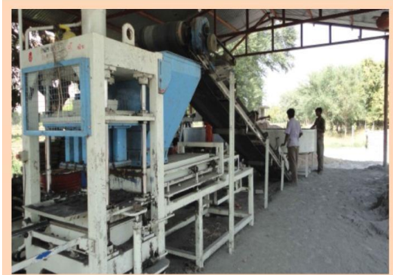
Fig 6: SET UP OF AUTOMATIC FLY ASH BRICK PLANT
