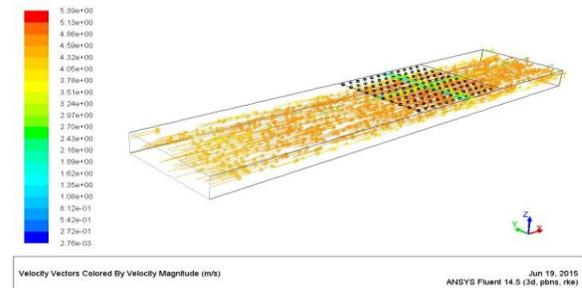
Fig.6 Plate-square-circular-p10-e-2-re-10000-velocity vector
