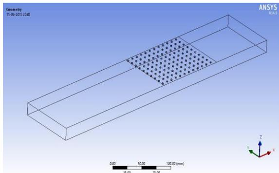
Fig.2-3-D domain SAH DUCT with combination of circular and square rib with e =2mm
