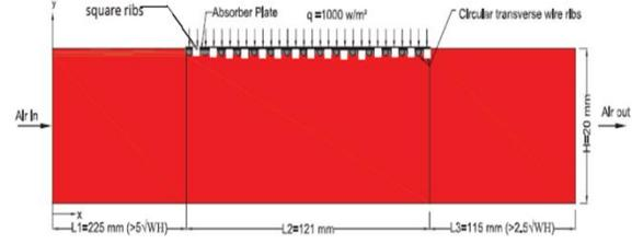
Fig.no.1 Computational domain for solar air heater with combination of Square and Circular ribs
