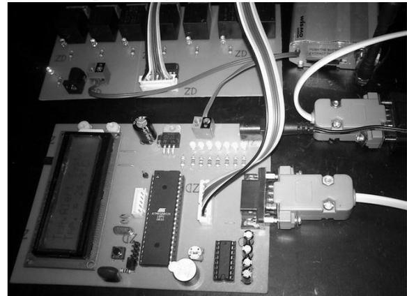
Fig 3: Room temperature monitoring system
