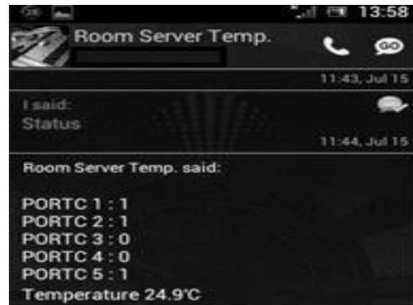
Fig 4: System testing with Status command
