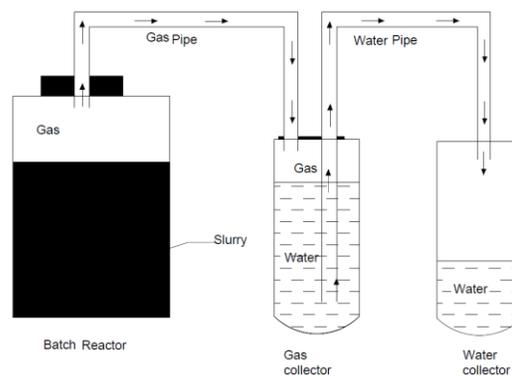
Fig. 1: Schematic Representation of Experimental Setup
