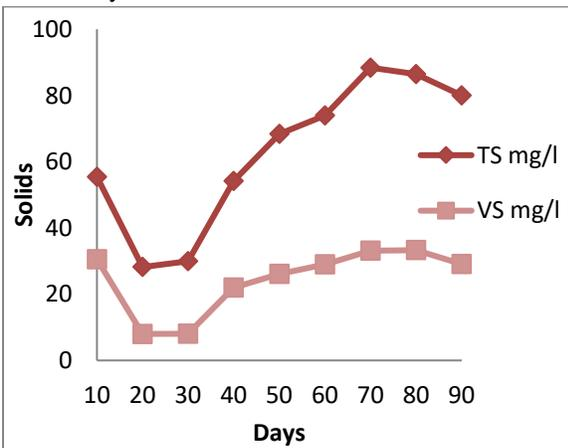
Fig. 3: Variation of TS & VS for Sewage sludge as Inoculum
