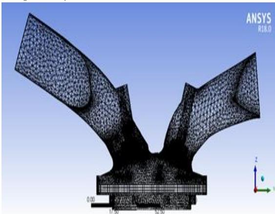
Figure 3.4 Meshed Geometry for Cold Flow Analysis
