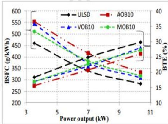
Figure 2.1 Changing of BSFC and BTE curves with power output.
