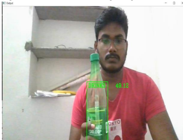
Fig.no : : Bottle detected and bounding boxes drawn around the detected object along with the confidence
