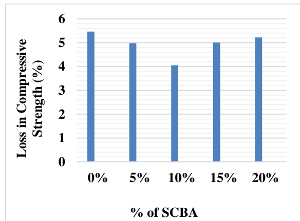
Fig. 4 Compressive Strength Loss of Concrete Specimens Subjected to Sulphate Attack
