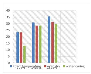
From the chart above we can easily make that the cube which are kept at room temperature acquires higher strength and also the cube which are kept for over drying achieve the target strength but the cubes which are kept for water curing fails to achieve target strength.
