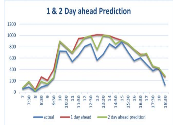
Figure 4.3: Comparison of actual and predicted values of solar irradiance for 1 and 2 days ahead prediction
