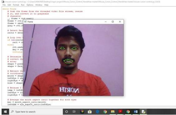
Figure 2: Eye Detection using Haar-Cascade Algorithm
