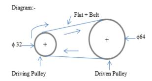
D  $\rightarrow$  Diameter of driven pulley  $\rightarrow$  64mm
