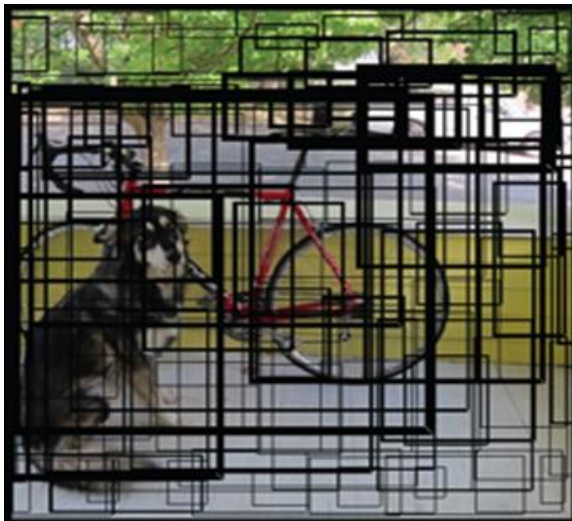
Fig. 3 the higher the confidence score, the fatter the box is drawn
