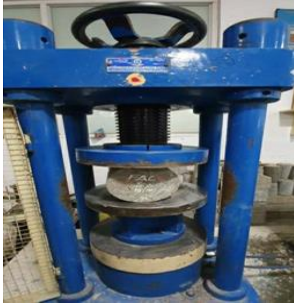
Fig: - Split Tensile Strength Test
