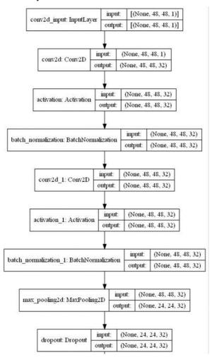
This is the flow of the first layer of the model. Here 32 is the number of filters that are eventually reduced when using max pooling. (3,3) is the size of the kernel. And the padding has been kept the "same" to protect the dimensionality of the volume. And the activation function used here was "elu".
