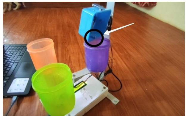
Figure 10: Metal waste detected and falls into respective dust bin i.e. Metal waste bin
