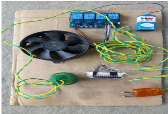
Fig- Connections of Google Assistant- controlled Home automation
