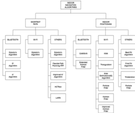
Figure 1: Indoor Navigation Algorithms for Shortest Path and Indoor Positioning
