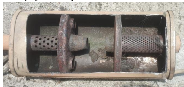
Fig 1: Hyundai Zen muffler cut section
