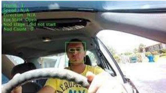
Figure 2: Successful Initial Face and Eyes Detection.
