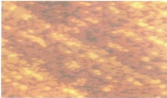
Figure 11, Atomic resolution 10x10 nm 2 constant height scan for 0.65 ML Fe coverage on the reconstructed Au (001) -hex taken at VB=2mV and I=3 nA.
