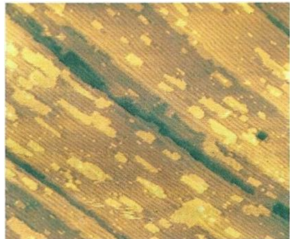
Figure 7, 100x100nm 2 scan on the topographic mode for 0.2 ML Fe coverage on the reconstructed Au (001)—hex surface, VB=3mV, I=1.2 nA.
