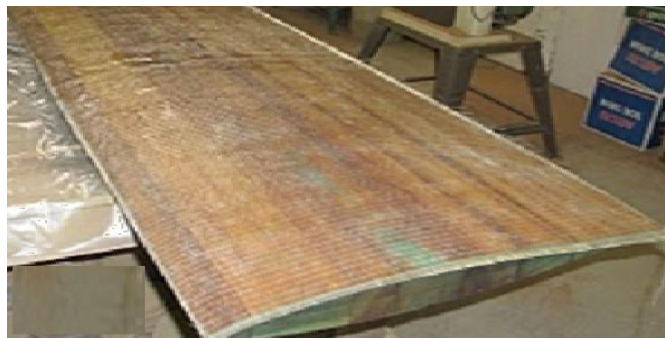
Fig: 1 Manufacture of the glass /epoxy composite beams From the above laminate beam prepare the test beam as per following dimensions as shown in fig.2.
