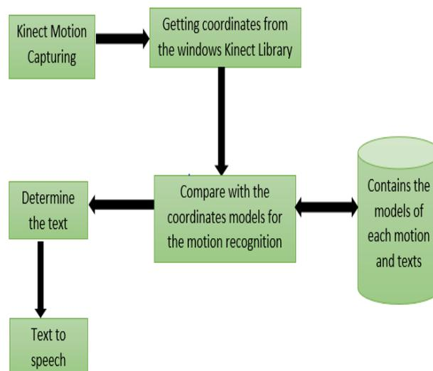
Fig 2. High level architecture of the proposed system
