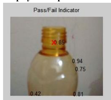
Fig12: Display the output of without cap bottle
