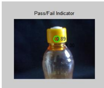
Fig9: Display of output with no defect
