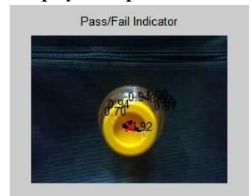
Fig11: Display the output of Defected bottle
