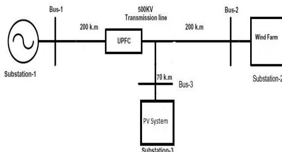
Fig: 2 Simulated transmission system.
