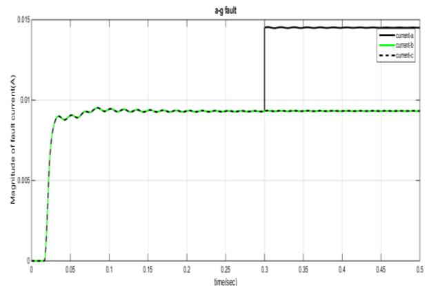
Fig:4 Current waveform when fault is applied at 0.3sec
