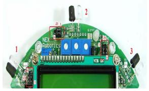
White line sensors are used for detecting white line on the ground surface. White lines are used to give robot sense of localization.
