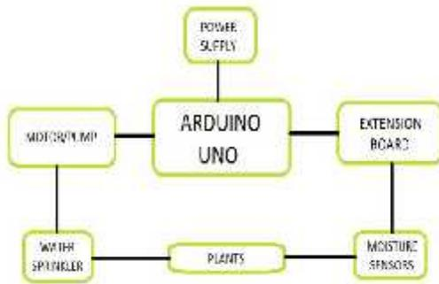
This project uses Arduino Uno to controls the motor. Follow the schematic to connect the Arduino to the motor driver, and the driver to the water pump. The motor can be driven by a 9 volt battery, and current measurements show us that battery life. The Arduino Board is programmed using the Arduino IDE software. The moisture sensor measures the level of moisture in the soil and sends the signal to the Arduino
