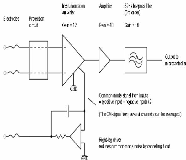
Figure3. Simplified block diagram of the Modular EEG amplifier
