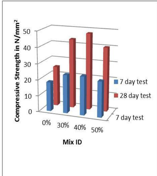
Fig III Bar chart showing the compressive strength of concrete
