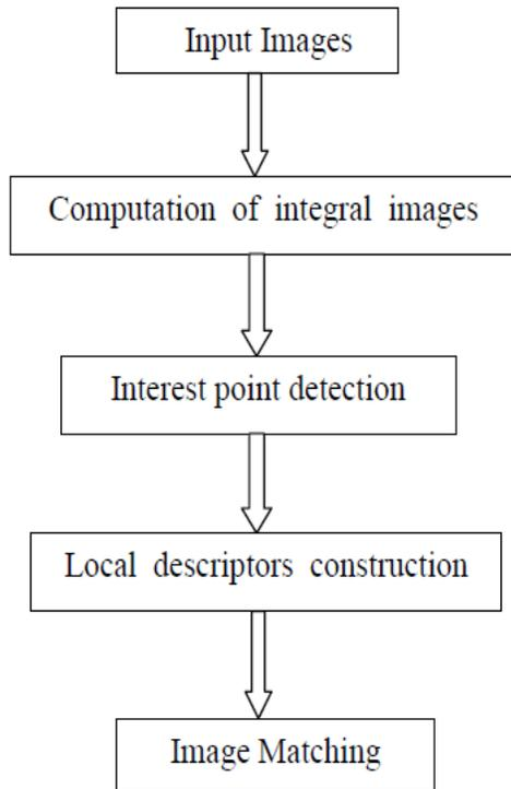
Fig SURF feature detection algorithm<sup>[13]</sup>
